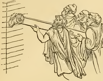
Roman Battering-ram worked by hand.
